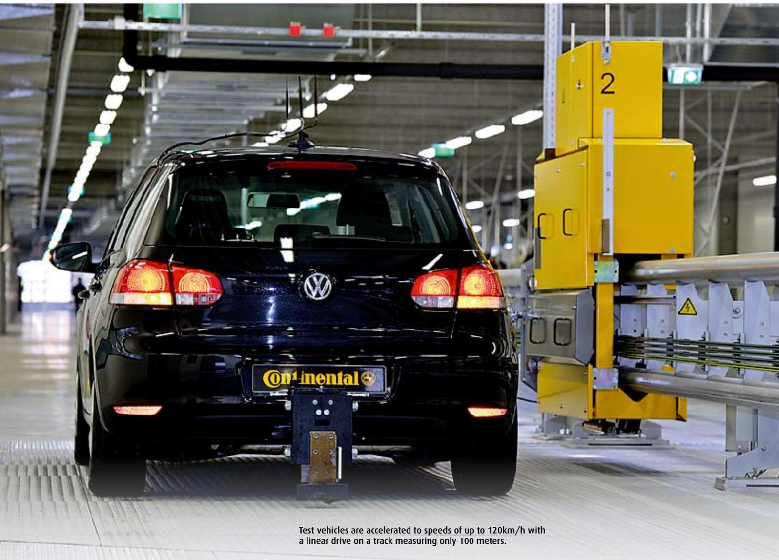
Test vehicles are accelerated to speeds of up to 120km/h with a linear drive on a track measuring only 100 meters.
