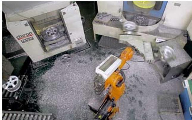
The mechanical processing of the blanks takes place in numerous automated CNC control systems.
