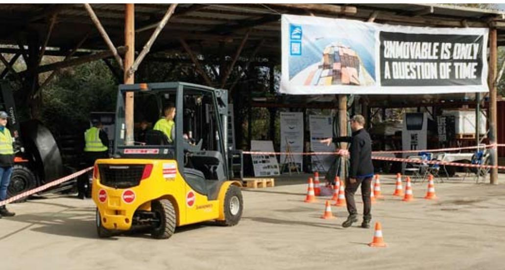
When using forklifts, the guests first had to get used to steering via the back wheels.
